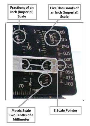
To gain resolution divisions on all scales of the Jr. Tri-Gauge are fine. Conversely these scales are linear, so estimating half measures in practice is acceptable.
